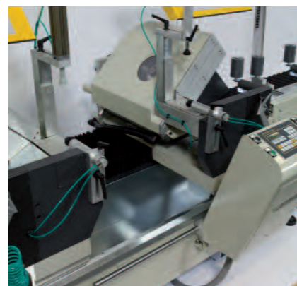
The frontal side is equipped with a wide chips collector and the guides are protected by a bellows
