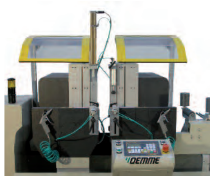
Brushless motor with sensor on magnetic strip ensures fastness and high positioning precision of the movable head
