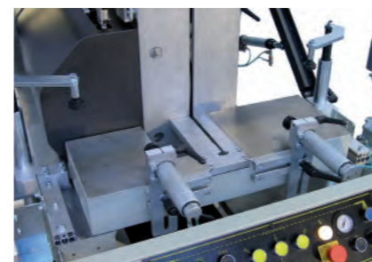
Automatic self-unlocking of the pneumatic vices with different working pressure when the carter opens, allows a quick cutting operation
