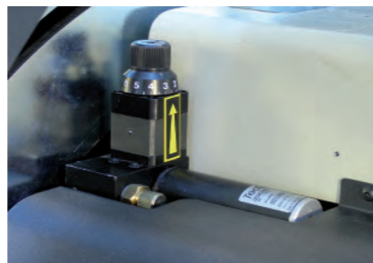
Valve for blade feed speed adjustment allows to suit different cutting possibilities according to the material specifications
