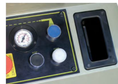
Two side pockets give a comfortable support to the operator's fingers while cutting off
